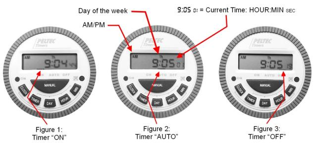
5. Press the "MANUAL" button until the small indicator line on the display is above "AUTO" (Figure 2). This allows the unit to work at intervals as set on the timer.
